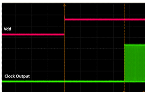
Figure 17. Startup Waveform vs. Vdd
