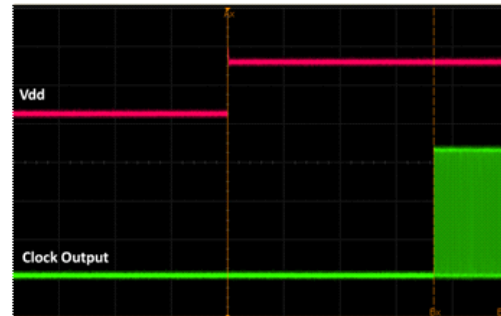
Figure 17. Startup Waveform vs. Vdd
